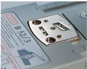
Bypass system: Staple ends are inversely bent away from each other. Advantage: Staples with long legs can also be used to staple thin stacks of paper.
